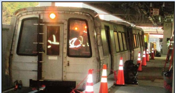
ON THE PLATFORM: The clearance car runs through the Wiehle-Reston East Metrorail Station platform on the outbound track. Photo by Denny Ondo, Dulles Corridor Metrorail Project
